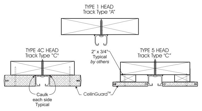
D. In **Type 4C** heads install CeilinGuard® head trim at each side of track with No.8 x 2¼" flat head screws. Use No.6 x 1½" flat head screws for **Type 5** heads. Great care shall be taken to assure a level surface (no side tilt) for SonicSweep™ (sweep seal) material to contact without binding.
