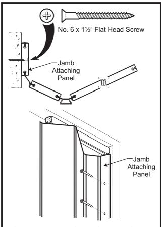
Place & Secure Jamb Attaching Panels
