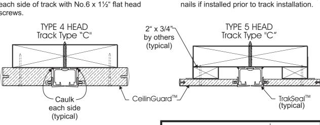
D. On Acoustical models Type 4C heads install CeilinGuard® head trim at each side of track with No.8 x 21/4" flat head screws. Use No.6 x 1<sup>1</sup>/<sub>2</sub>" flat head screws for Type 5 heads. Great care shall be taken to assure a level surface (no side tilt) for SonicSweep<sup>™</sup> (sweep seal) material to contact without binding.
