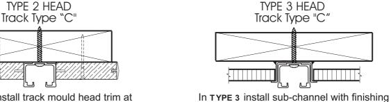
In TYPE 2 install track mould head trim at each side of track with No.6 x 11/2" flat head screws.
