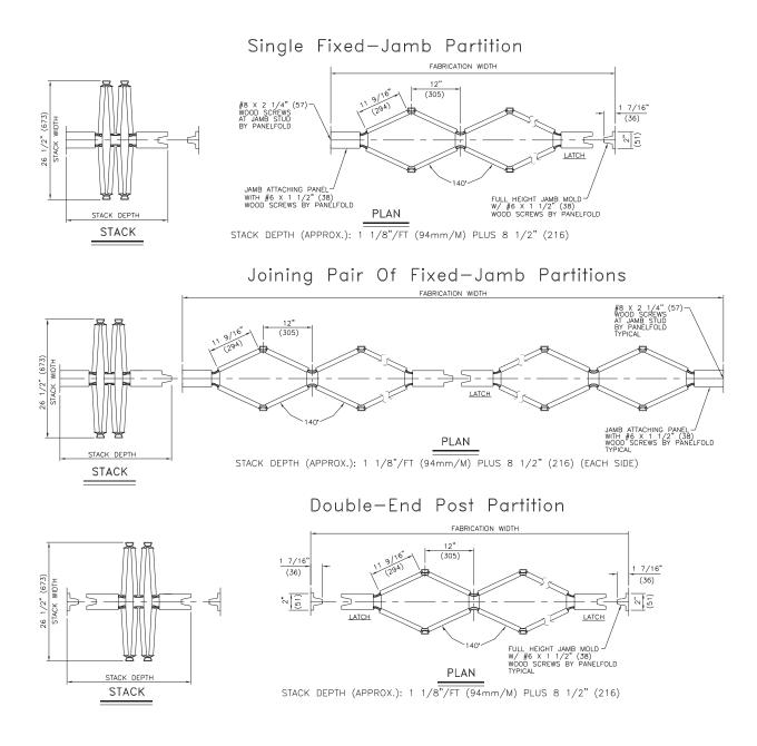
All dimensions shown in parentheses are millimeters. Scale: N.T.S.
